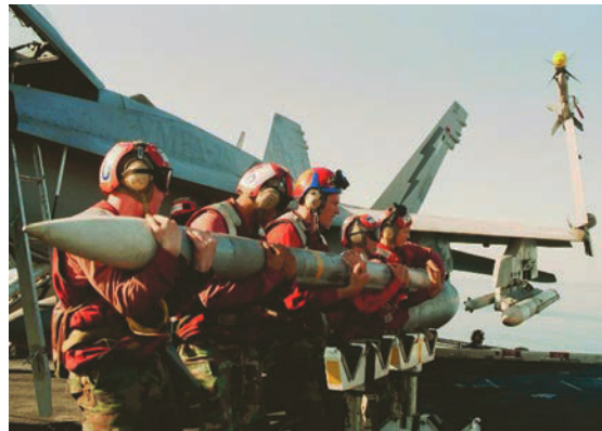
Official Marine Corps photo Ordnancemen on board the USS Theodore Roosevelt (CVN 71) arm a F/A-18 Hornet from Marine Fighter Attack Squadron 251 with an AIM-120 advanced medium range air-to-air missile.
