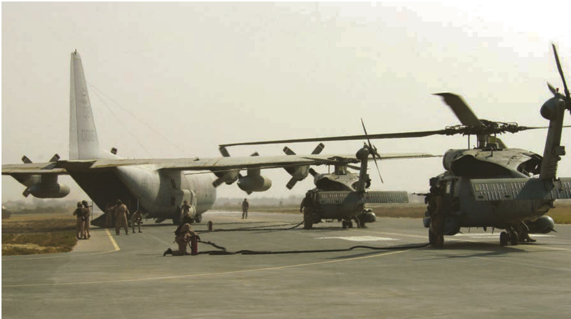
Photo by TSgt Scott Reed, USAF Defense Imagery, VIRIN: 011109-F-4884R-010 A KC-130 Hercules aircrew from Marine Aerial Refueler Transport Squadron 352 performs a rapid ground refueling of two Navy Sikorsky SH-60 Seabawk helicopters at Shabbaz Airbase in Jacobabad, Pakistan, on 9 November 2001.
